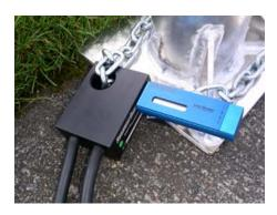
Secure the Road Runner<sup>™</sup> to a solid sign post or other similar roadside object to prevent theft and vandalism. It is best to place the unit so it is out of plain view or away from the road to deter tampering.
