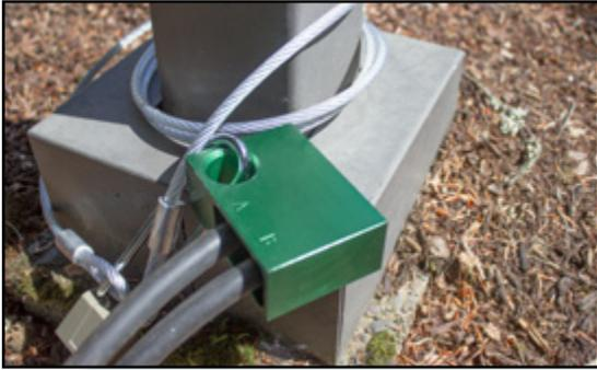
Field set-up is a breeze in all weather and space conditions. Set road tubes for counting one or two lanes, attach them to the Road Runner, and lock it on the roadside. The unit is always counting.
